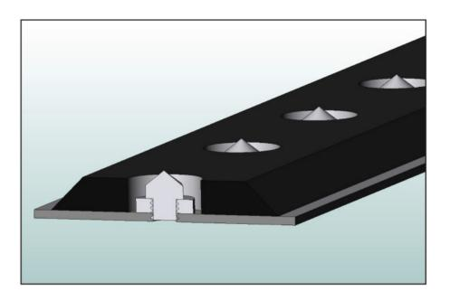
Replaceable conical shaped spikes are threaded into a special feed slat insert.
