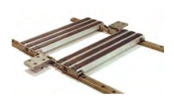
High friction Posi-Feed bed featuring aluminum slats with replaceable steel-backed rubber inserts. Precision feed chains ride on hardened steel Double-Vee rails.
