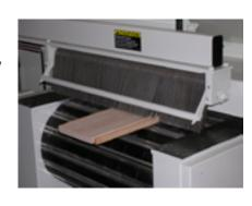
Direct coupled feed drive with variable frequency speed control and overload protection. Feed rates 30-225' per minute, higher rates optional.
