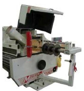
Standard removabe sleeve and saw spacers provides high accuracy.
