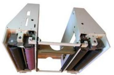
Heavy duty, high yield pressure head mounted on cast iron "U" Column features air loaded rolls providing smooth conveyance of both surfaced and rough stock material.
