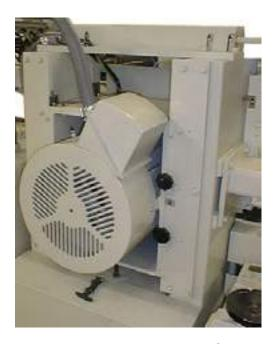
Direct drive arbor motor for maximum efficiency without belts to tension or replace.
