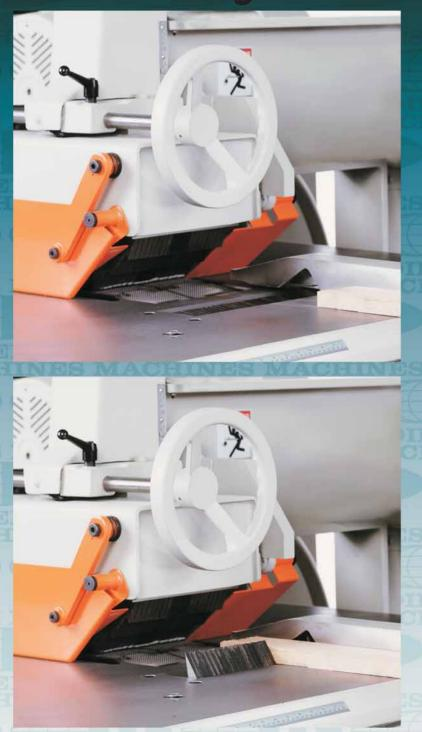
Automatic raising and lowering of the lower kickback fingers is available as an option on all Diehl rip saws, and is especially recommended for operations where shorter stock is being processed. The feature provides two alternative methods to sense stock presence and lower the fingers below the worktable for easier and faster feeding.
