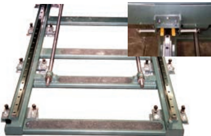
Machine Base: Heavy wall structural steel weldment with linear rails and air actuated position lock
