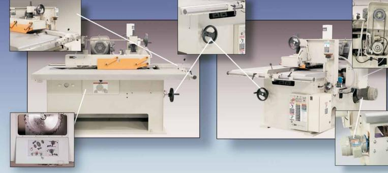
The front view illustrates access into the electrically interlocked saw pit area, the dual anti-kickback finger system, pivoting pressure beam side guard and the standard rail mounted stock guide. The machine's back side is shown with the arbor drive housing removed to depict the automatic arbor brake and the "Poly-Vee" arbor drive belt. Also shown are the adjustment handwheel for positioning of the saw blade for varying thicknesses of material; and the 5 HP feed chain drive assembly.
