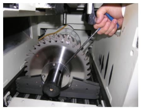
TwistLock saw collars are manually locked into the desired position with the supplied "T" handle wrench providing positive locking power. Great for narrow rip application requirements.
